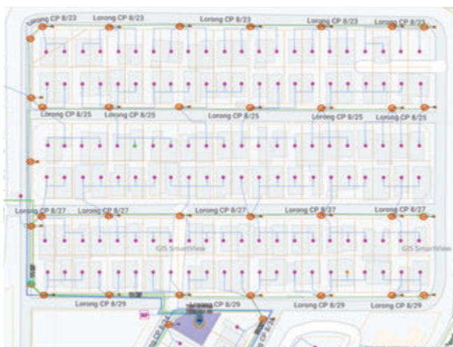
Figure 4: Sample GIS data on asset topology and network connectivity connections from distribution substations to customer meters
