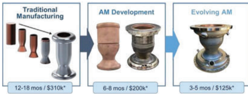
Figure 2: The evolution of traditional manufacturing to Additive Manufacturing 4
