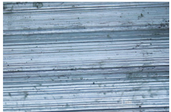
Figure 7: Diagram of Titanium alloy with highest surface roughness using PCD insert
