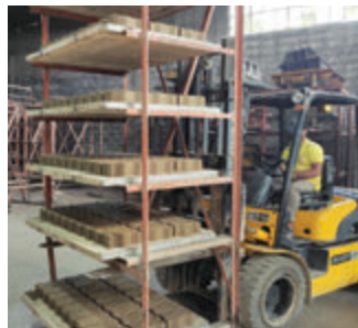
Figure 3: Carrying to the storage place for curing
