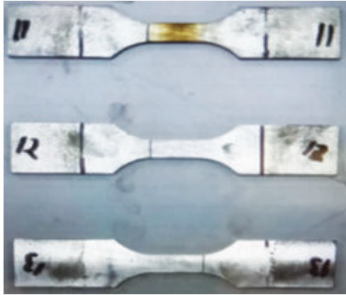
Figure 6: Specimens fracture under tensile testing
