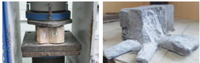
Figure 5: Compressive strength testing of concrete paving block units (a) compressive strength test setup (b) typical rupture for a whole paving block
