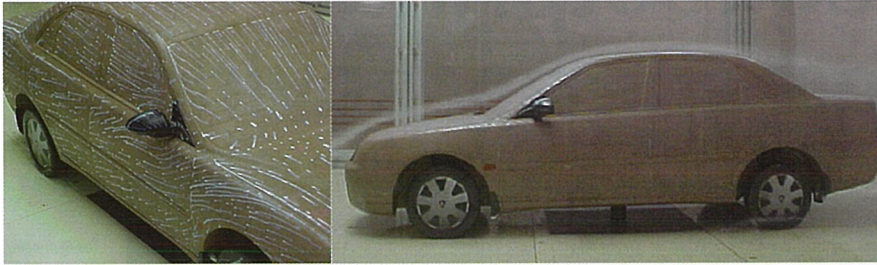
Figure 10: Flow visualisation using smoke and oil
