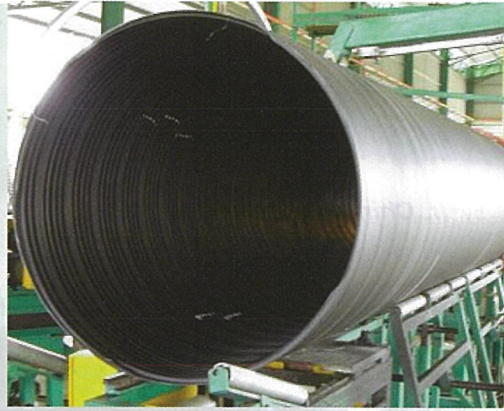
Rib Loc HDPE Pile Jacket Through Reversed Winding Process
