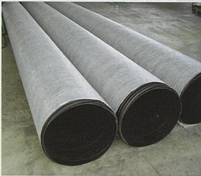
Rib Loc HDPE Subsoil Pipes Diameter of 525mm with a Layer of Geotextile as a Soil-Water-Separator
